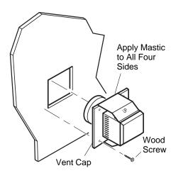
Figure 23 - Installing Horizontal Vent Cap
